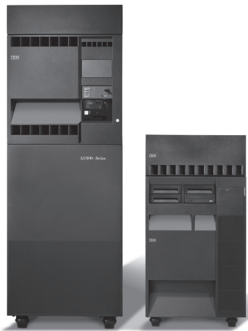
Figure 1.15. AS/400e server 840 and e-server 840-SBI.
