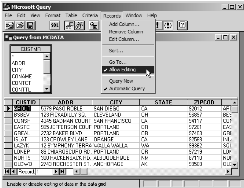
Figure 3.20: You can edit live iSeries data by selecting the Allow Editing option.
