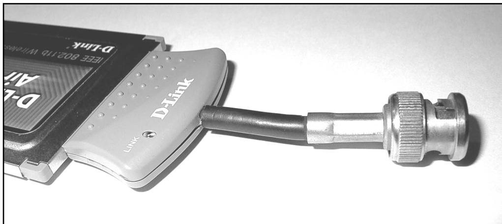
Figure 10.11 The Finished Hack: D-Link DWL-650 with External Antenna Connector
