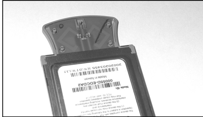
Figure 10.7 Inside the Antenna Compartment
