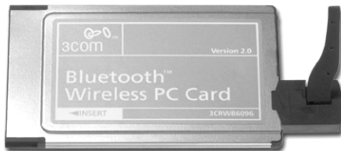
Figure 1-3 3Com's Wireless Bluetooth PC Card fits into a notebook's PC Card slot, letting the user communicate with other Bluetooth products, including PDAs, printers, digital cameras, and other enabled computers.
