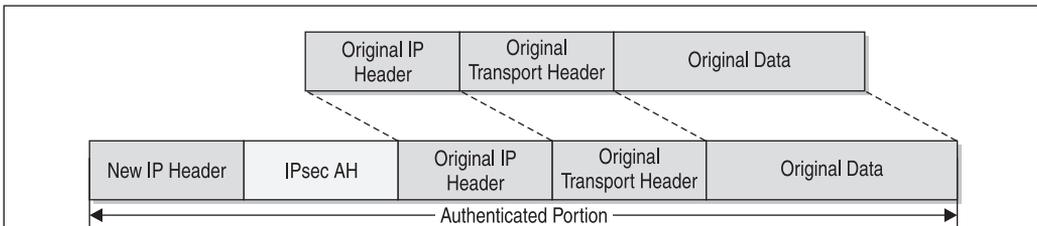
Figure 5-8. AH tunnel mode
