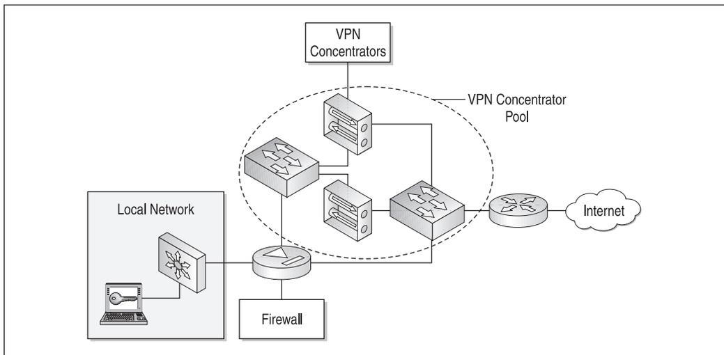
Figure 5-3. Simple VPN redundancy
