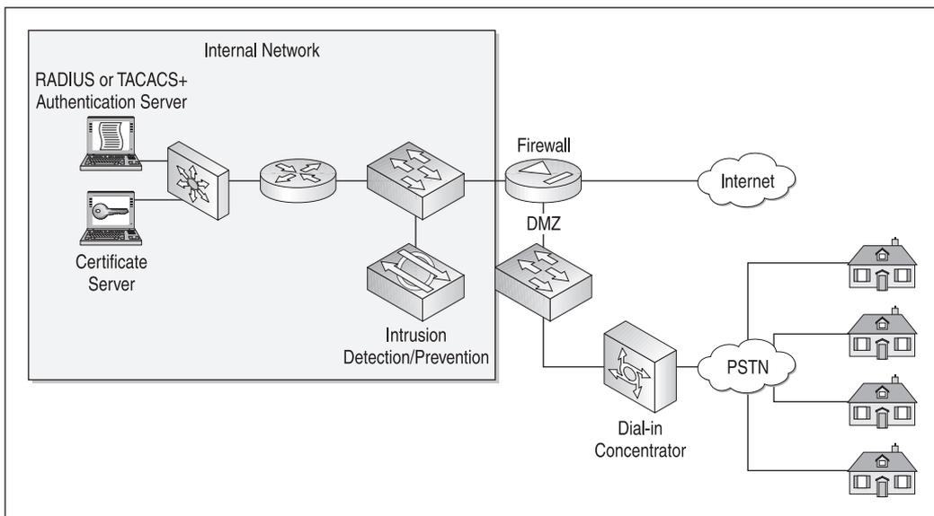
Figure 5-10. Dial-in access network design
