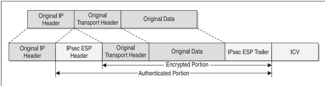
Figure 5-7. ESP transport mode
