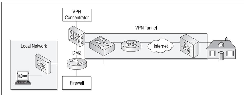
Figure 5-1. Basic remote access VPN
