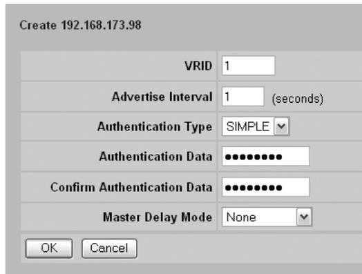
The final step is configure VRRP on the interface by going to the Routing | Interfaces | Routing Interfaces screen and clicking Configure. This will take you to the Routing | Interfaces | Routing Interfaces --> Configure VRRP screen, as shown next. Configure your system to enable VRRP, and with the appropriate master status. If this is the master device, make sure you have selected the appropriate group, selected to serve as the master, and enabled the administrative state.
