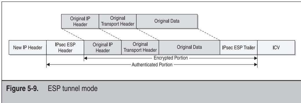
**Figure 5-9.** ESP tunnel mode
