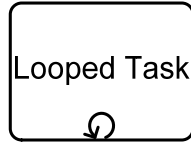
Figure 7-3—A Task with an internal loop
