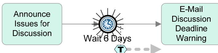
Figure 8-34—When the Timer is triggered, the token continues
