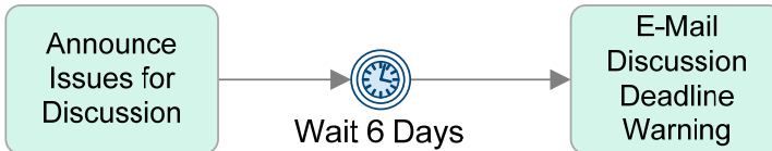
Figure 8-31—A Timer Intermediate Event creating a delay in the Process
