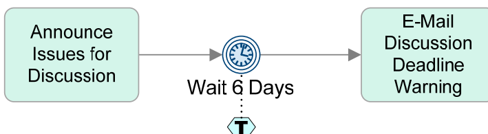
Figure 8-33—The token will be delayed until the Timer is triggered
