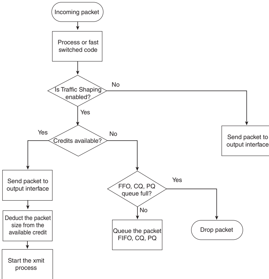
Figure 15-28 Traffic Shaping Flowchart
